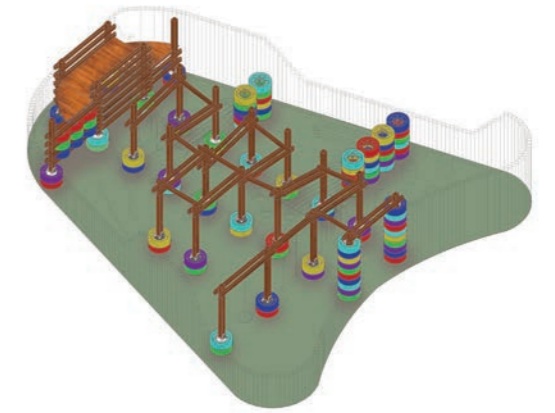
Partitions - Reclaimed materials - timber boarding & tyres
