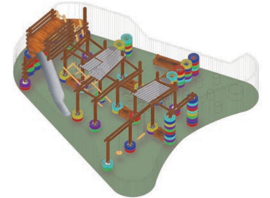
Play equipment - Reclaimed bamboo and steel slide
