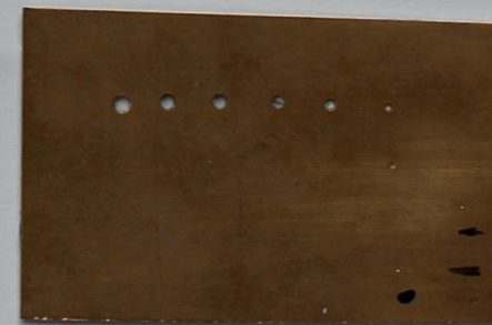
SCRAP METAL - used to test out the Disc Cutter punch sizes for the dimension of the gold coin.
